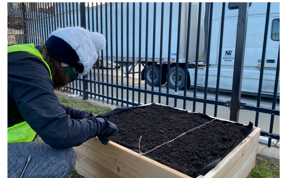
Image → Installing twine sampling grid on soil plot
